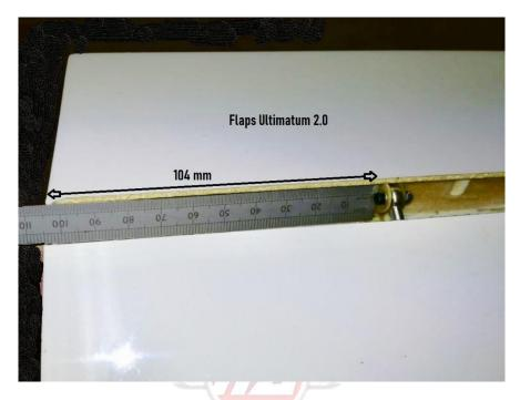
$\Phi$  During assembly, do not deflect the flap more than 70mm, the hinge could be damaged and will not be covered by the warranty  $\Phi$
