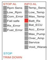
"Temp\_Sens" indicates a temperature probe failure.
