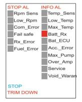
Stop Alarms appear when the problem was significant enough that the ECU command the turbine to stop during a run cycle.
