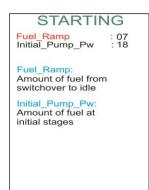
There are only two adjustable parameters in this sub-menu, "Fuel Ramp" values and "Initial Pump Pw".
