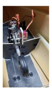
Mount the back door servos on the carbon laminated wood.
