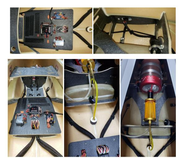
We provide an electronic tray where you can install the electronics (Receivers, ECU, Landing Gear Control, Gyro, and batteries. This tray is made of wood with laminated with carbon fiber. Check your radio manufacturer recommendations for the setup of the receivers to avoid any radio signal interference.
