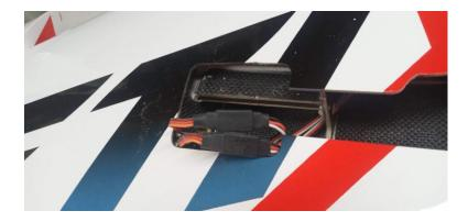
Space is provided where the mechanics for the retracts are installed to accommodate the connections between the wire harness (extensions) and the retract/brake system connectors.
