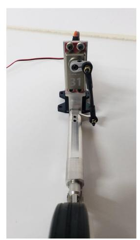
Mount the servo onto the servo plate, as shown in the pictures. The length of the servo arm should be 20mm.
