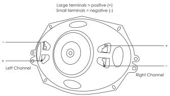
Wiring our RetroSound<sup>®</sup> dash speakers in series so the amplifier sees an 8 ohm load:
