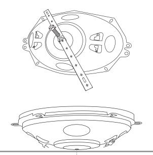
Install bolt into hole in back of magnet
