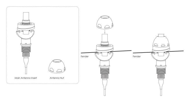
6. Thread the antenna adapter into the bottom of the antenna mast. The fine threads go into the mast. Then thread the nut onto the end. Do not over tighten.
