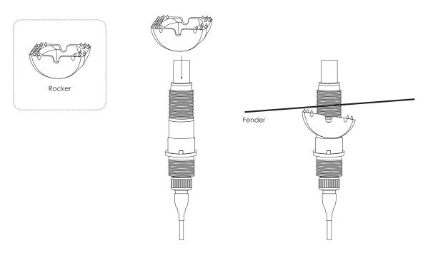
4. Once the antenna assembly has been placed through the antenna hole, place the rubber gasket and slant bezel over the main antenna insert from the top.
