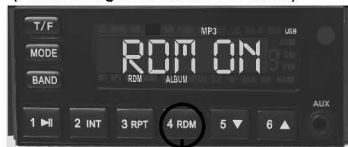
Press "4" (RDM) to allow the unit to randomly play tracks on your USB drive (Press RDM again to cancel this mode) (Note: Random mode will access any file located in or outside of folders when in this mode)
