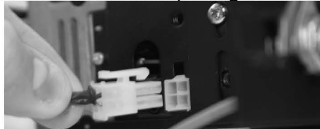
Plug Shaft into Side of Main Unit
