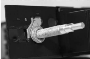
Mount Shaft to Bracket
