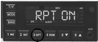
Press "3" (RPT) to Repeat the currently playing track (Press RPT again to cancel this mode)
