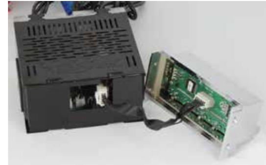
Connect the ribbon cable included with the radio body to the radio face.
