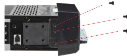
Attach the radio face to the radio body using the radio face mounting screws included.
