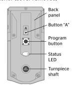
Note: When the cover is removed, the turnpiece shaft can be used to manually lock and unlock the door.
