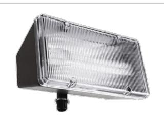
High quality polycarbonate PL floodlight. Supplied with one, two or three 13 Watt twin tube compact fluorescent lamps. Adjustable swivel mounting arm with 1/2" thread. Lamps supplied.
