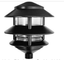
Rugged die cast aluminum 6" diameter housings. Threaded, gasketed clear glass globe for durable weatherproofing and easy relamping. 1" long, 1/2" threaded nipple included for easy mounting. 75 Watt max. Incandescent lamp not supplied. Fluorescent lamp supplied.
