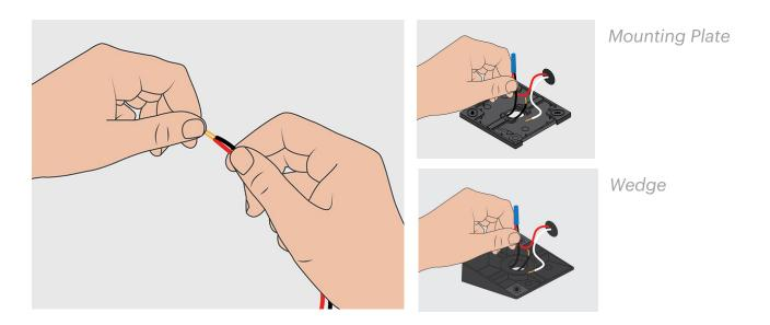
Using pliers or a crimping tool, crimp the dolphin connector very hard, starting at the top of the connector downwards. Repeat this process for the other two wires.
