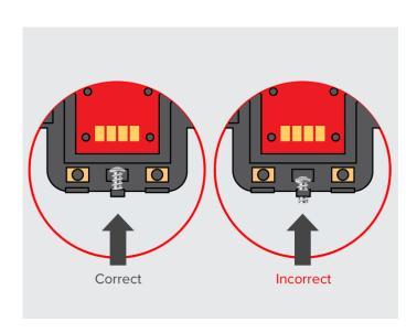
After you've checked the security screw, align the Doorbell Cam over the top lip of the mounting plate/wedge, then push the bottom of the Doorbell Cam firmly.
