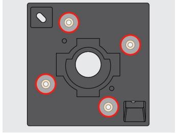
Take the mounting plate and place it over wedge, aligning the same holes to the gold screw holes. Run the wiring through the large-middle hole of the wedge. Note the "UP" arrow, it should face upwards. Then take two of the three screws that you set aside earlier and use them to attach the mounting plate to the wedge.
