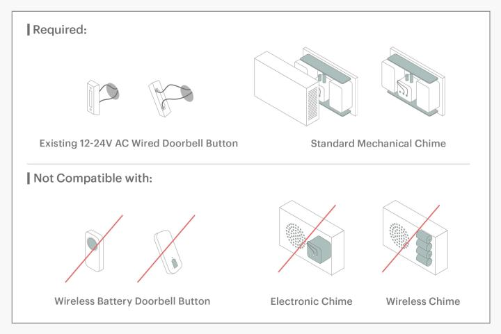
If your existing doorbell has a speaker, it's a digital chime. If it has a mechanical mechanism (usually in the form of two pistons that strike metallic keys), it's a compatible mechanical chime. You'll need to ensure that your doorbell is getting 16-24V from the transformer.
