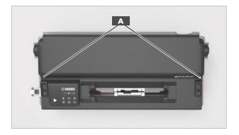
2 SLIDE THE TRIGGERS AND LIFT HEAD UNIT Slide the triggers down as shown below.
