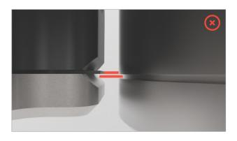
If the indicator tab of the **Alignment Tool** is aligned with the groove on the **Alignment Ring** (as shown below) skip to step 8.
