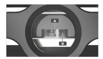
Ensure you are looking straight through the eyepiece directly above the indicator tab and groove. If you see the indicator tab side wall (C) when looking through the eyepiece, you are not directly above the indicator tab and groove. Adjust your line of sight until you can no longer see the indicator tab side wall.
