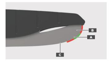
When the intersection zone is a curved surface (A as shown above) the **Grinding Ring** can safely initially contact the blade anywhere in this region (A).
