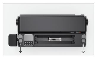
With the triggers slid down, raise the head unit and remove the contents inside.
