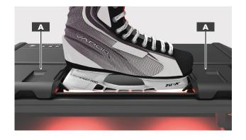
We recommend inserting the skate into the **Skate Clamp** with the toe pointing to the right. For most skate blades, this orientation allows for the greatest flexibility in **Grinding Ring** height adjustment. It is, however, acceptable to insert the skate with the toe facing in either direction.
