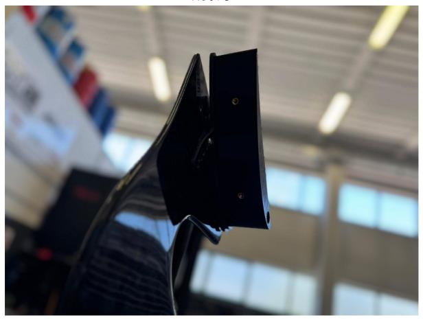
MOUNT BOTH SIDE BRACKETS AND CONNECT THEM TO THE WING BY INSERTING THE BRACKET INTO THE WING, USE THE SHORT SCREWS AND SCREW THEM THROUGH THE HOLES IN THE BOTTOM OF THE WING.
