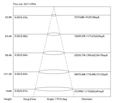
Note: The Curves indicate the illuminated area and the average ilumination when the luminaire is at different distance.
