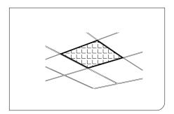
3. Put the lamp into the ceiling groove and make sure it is firm.
