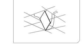
2. Make sure the power is off before installation. Open the bottom hole and connect the wires.
