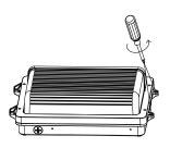
2.Use a screwdriver to remove the screws on both sides and remove the upper cover of the fixture.
