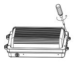
2.Use a screwdriver to remove the screws on both sides.
