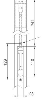
Flush bolt (FB6200) used at top and bottom of stile for locking purposes
