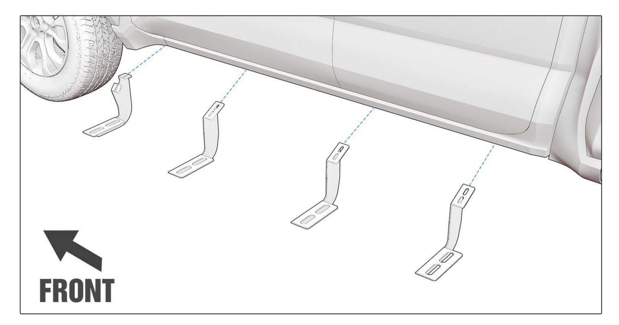
• First, there are six mounting bolts underneath the vehicle. Use a socket wrench to remove all of them. Repeat the same process on the other side.
