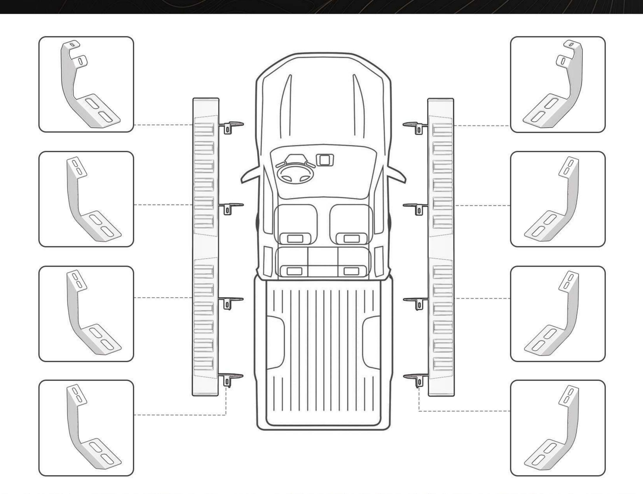
PREPARE ALL THE BRACKETS THAT NEED TO BE INSTALLED AND DISTINGUISH THE DIRECTION, AS SHOWN IN THE FIGURE.
