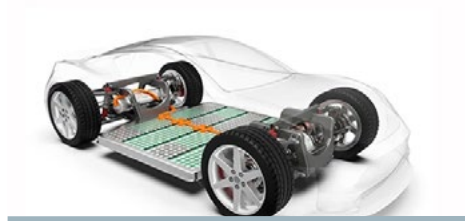
High Voltage Battery
