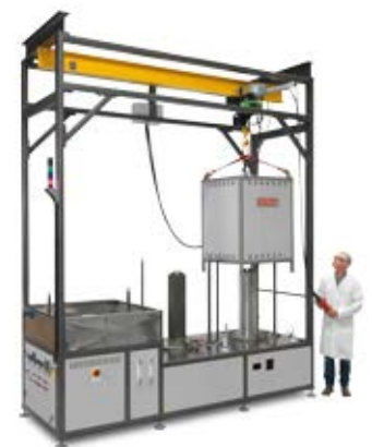
Top hat furnace system with twin retorts
