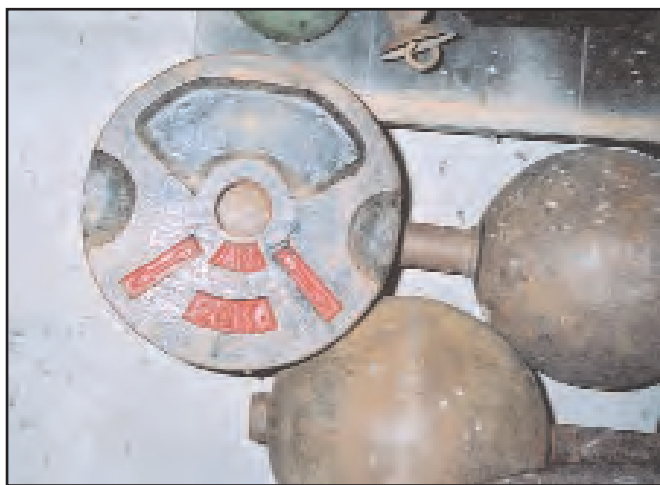
Roux 20 Kg Olympic plate with recesses on edges for fingers to slip under when lifting off floor.
