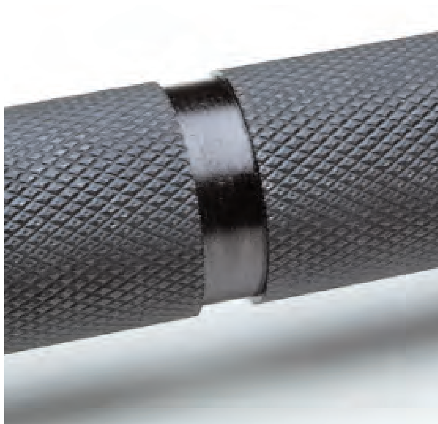
A bar showing a typical “suicide groove”. This cosmetic feature will weaken the bar at this point, and is often the precursor of bar failure.
