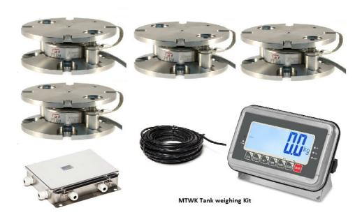
This Tank/ Silo/Hopper weighing kit is suitable for Tanks, silos & hoppers from 250kg to 120t capacity. The kit has four tank weighing load cell assembly with uplift protection. Load cells are sealed to IP68 protection and the complete assembly is made in stainless steel. The MI102SS indicator & junction box are IP66 rated.
