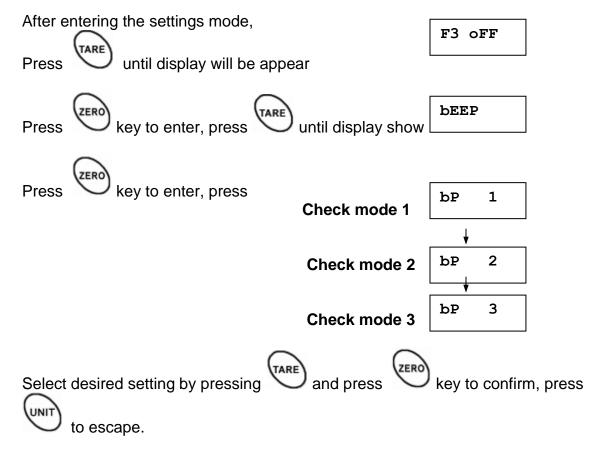
Note: The load weight must greater than 20 scale divisions for the check weighing operations.
