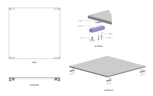
There is a load direction arrow at the loading end of the load cell (peel off the bar code label if arrow is not visible). Swivel foot is fitted from the opposite end of arrow direction, as shown in picture below.
