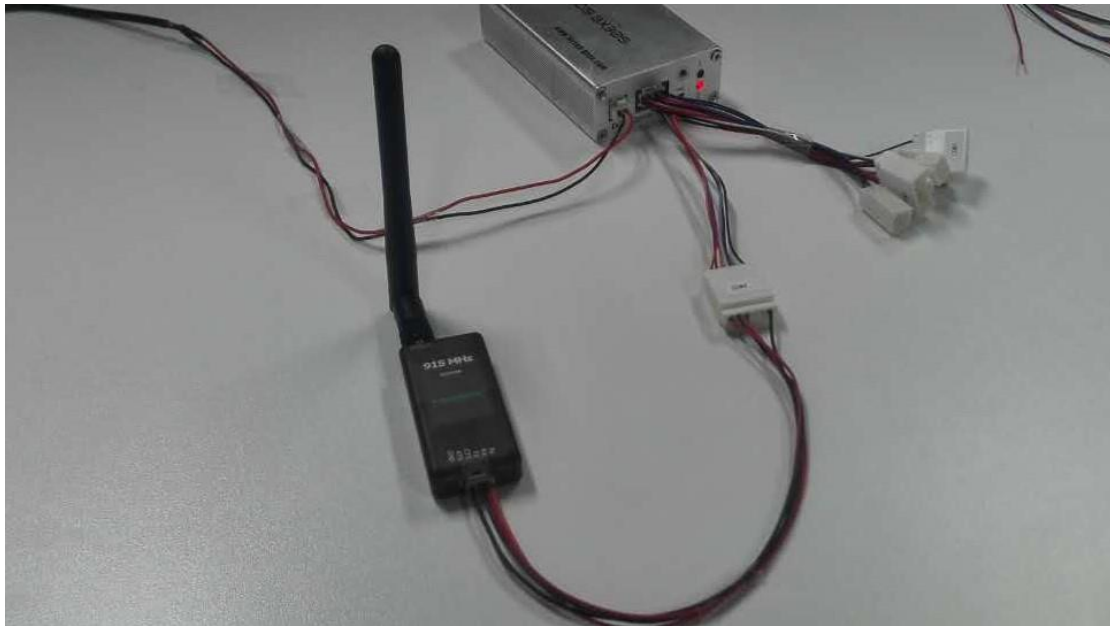
Figure 16 Connection between Pixhawk and Preci-BX306
