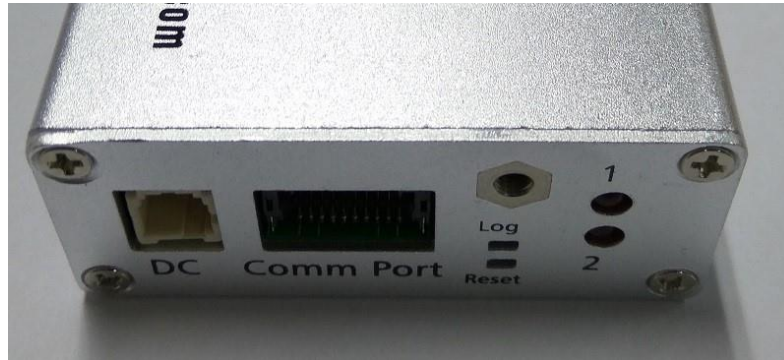
Figure 12 Power and communication ports
