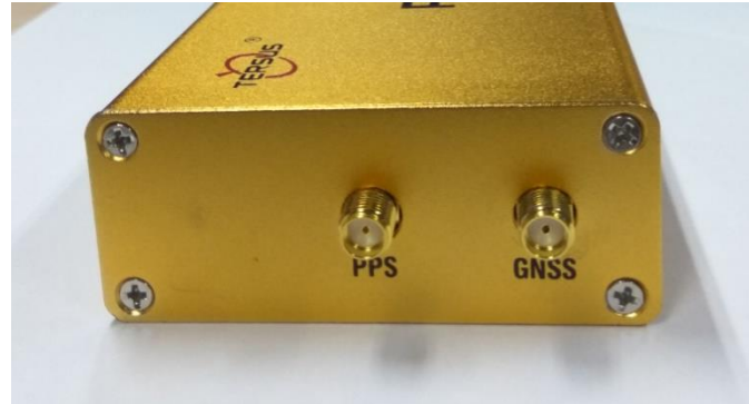
Figure 6 Ports at the left side of BX306 receiver V1.1
