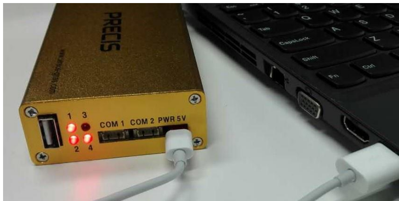
Figure 9 BX306 receiver powered via an USB port
