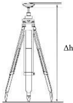
Figure 32 Demonstration of antenna height measurement
