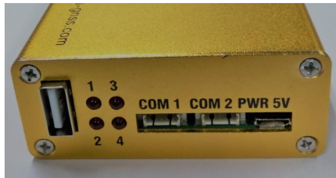
Figure 5 Ports at the right side of BX306 receiver V1.1
