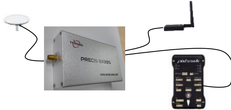
Figure 30 Demonstration of Integration with Pixhawk autopilot
