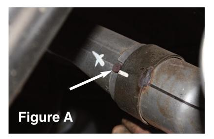
To fit 2007-'11 Jeep Wranglers, the pin (see arrow) on the stock pipe must be removed. Pin is easily removed with a hammer and chisel. Note this pin serves a purpose on the stock exhaust but is not required to install the Legato Performance Exhaust System.
