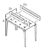
0.4 Assemble the remaining part A onto the open side. Once all nodes are in the right position, use a mallet to ensure they are firmly in position. Insert the dowels on the side with the A frame to secure the pieces.
