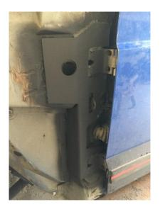
7. You must trim a small section off the Factory Fender. Use a cut off wheel or sanding disc to clearance the area shown in the pic below.
