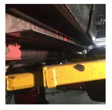
1. Using a cutoff wheel or plasma cutter, remove the factory rocker panel. Cut just behind where the sheet metal turns down past the door. It will leave a "lip" like in the pic
