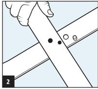
Step 2 - Align pin with pinhole to hold base in position.
