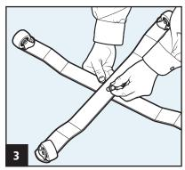
Step 3 - Insert bolt through both bases. Threads should be pointing up when base is upright.
