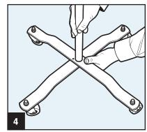
**Step 4** – Screw either end of pole onto threaded end of bolt.
