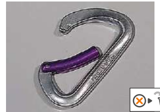
• Defective return spring
