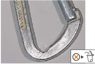
• Frame worn by the rope
