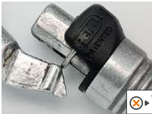
• Defective locking system
