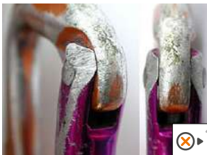
• Worn gate and frame
