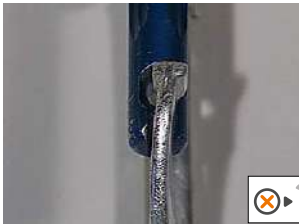
• Bad gate/nose alignment
