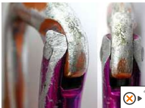
• Worn gate and frame
