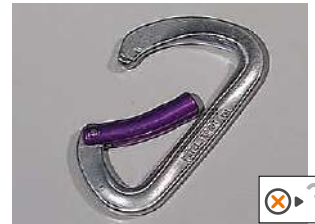
• Defective return spring
