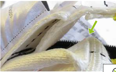
• No tearing of the energy absorber
