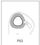
Check the condition of the fixed side plate (marks, deformation, cracks, corrosion, wear).
