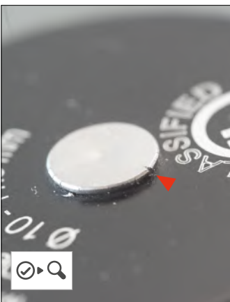
• Rivet slightly cracked
