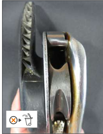
• Worn cam groove
