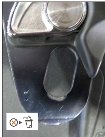
• Attachment hole deformed by a shock load
