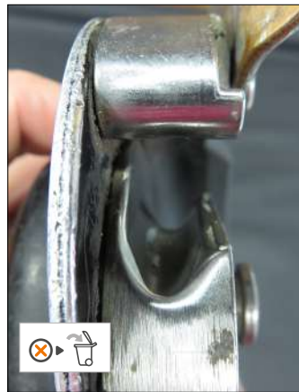
• Cam groove worn to wear indicator
