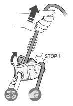
1. Pull on the climber-side rope; the device should lock the rope.
