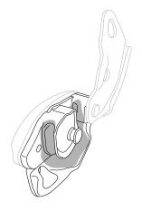
• Verify the absence of foreign objects (sand...) or lubricant on the rope channel.
