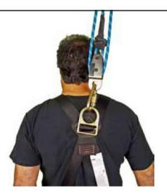
Apply firm tension on the safety rope to maintain a secure hold on the ring. Then pull the rescue rope toward you while holding the telescoping pole in place. This will cause the spring on the SureClip to compress causing the auto locking gate on the carabiner to close.
