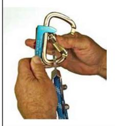
With the carabiner gate in the full open position, open the finger of the SureClip by pinching the finger against the main beam. This will open the jaws of the SureClip and allow you to slide the carabiner down through the jaws.
