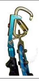
Continue pushing the carabiner down until it cradles into the spring, apply additional downward pressure until the gate clears the bottom of the jaws. Once the carabiner gate clears the jaws, release finger pressure to close the jaws and secure the carabiner. This completes the loading as shown on the left.
