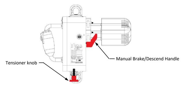
9. Once you are safely on the ground and sufficient slack has been taken out of the rope, then release the brake and you may now unclip from Ronin Lift.
