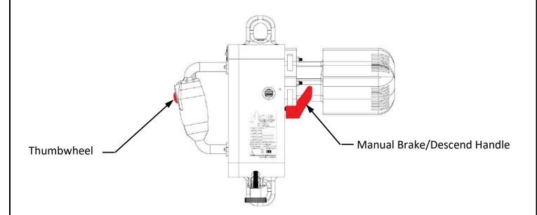
7. When descending its best practice to TAP the thumbwheel and then simultaneously pull the brake handle down. This will help to preserve your rope. (Note: If you pull the brake handle open and do not descend or descend very slowly, then turn the Red Tensioner Knob to the Right (clockwise) 1-2 turns, until you start to descend. This is due to the tensioner knob being too tight for the weight you are lifting.
