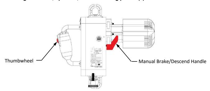
6. When ready to stop ascending release the thumbwheel switch. (Note: The brake is always engaged, while ascending. Once you stop your ascent the Ronin will automatically brake in that spot).
