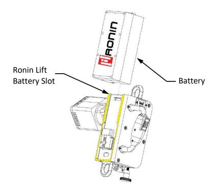
2. Drive the battery down with enough force to mate the connectors.
