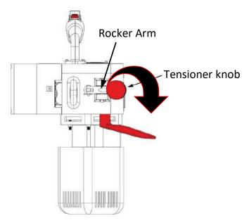
Note: Remove any tape or markers from the ends of the rope, before inserting into the Ronin Lift. Make sure your ends are burnt and No inner core is exposed.
