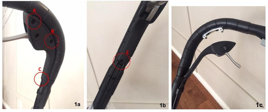
2. Lace grip onto stroller handle bar as normal (see lacing guide here: <a href="https://www.luxandleather.com/pages/how-to-attach-grips">https://www.luxandleather.com/pages/how-to-attach-grips</a>). Lace over the metal screw assembly, making sure not to pull the leather over it. Tie and cut off excess lacing thread once cover is fully laced and tightened.
