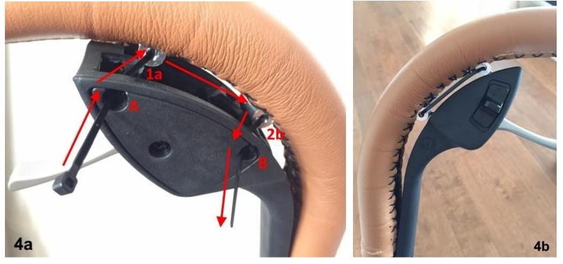
5. Push hand brake assembly firmly onto the metal screw assembly and into the handle bar. Be sure the zip tie is not coming out from the front of the assembly (4b). Connect the zip tie together and tighten, and cut off excess (5a).
