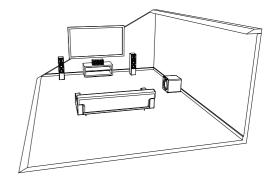
Side Wall Placement: Side wall placement is less frequently used but can be an effective subwoofer location for excellent accuracy and output.
