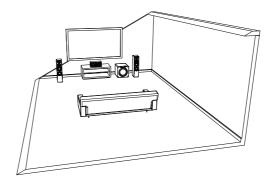
Front Placement: In between or to the side of the front channel speakers often results in the best blending with the main speakers and center channel and minimizes localization effects.
