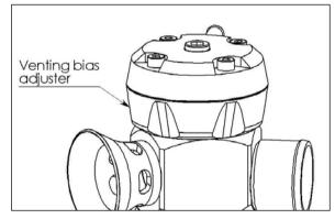
50/50 is reached. As you turn the adjuster further clockwise, the recirc port is fully open and the trumpet port will begin to close. When the adjuster reaches the maximum clockwise position, the trumpet is completely closed, and the valve will operate like a factory recirculating bypass valve.
