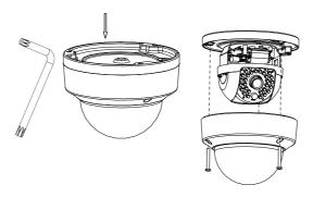
3. Fix the mounting base on the ceiling with screws.
