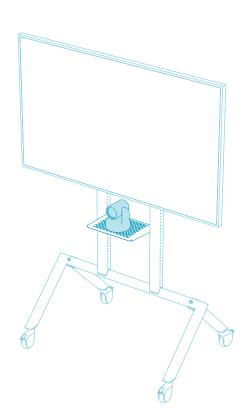
Note that the center slots include 1/4" clearance holes for camera mounting.
