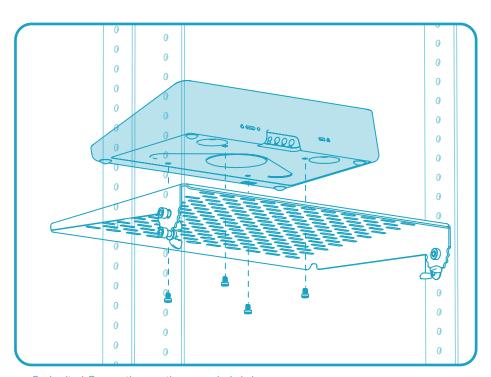
For Logitech Tap, use the mounting screws included inside of Tap's underside panel. For Neat Pad, use the M4 mounting screws included in Neat Pad's packaging.
