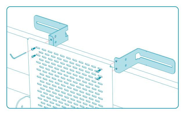
**STEP 4**Fasten the wingnuts and install the soundbar.
