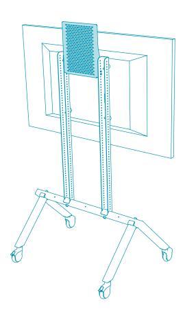
Install the soundbar-mounting brackets to the hole pattern of Device Panel as needed to create alignment with your soundbar's mounting points. Note that the brackets can be installed closely to each other if needed.
